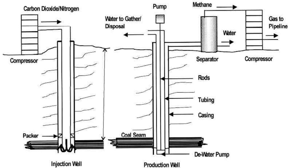
Figure 1. Gas is injected in one well and methane is recovered in another well. (After O.H. Barzandji, K-H.A.A. Wolf, J. Bruining, *Combination Of Laboratory Experiments And Field Simulations On The Improvement Of Coalbed Methane Production By Carbon Dioxide Injection*, Delft University of Technology Second International Methane Mitigation Conference, Novosibirsk, Russia, June 18-23, 2000).
